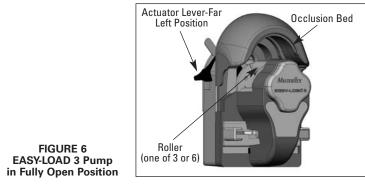
To unload tubing from the pump, turn off the drive. Then open the pump by moving the actuator lever counterclockwise (left), as described above. The pump will automatically open the tubing retainers, as well as lifting the occlusion bed away from the tubing. Then pull the tubing away from the pump front.
