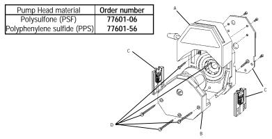
D. Mounting hardware for I/P EASY-LOAD pump heads.
