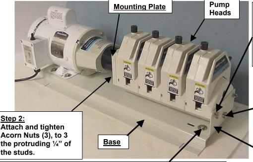
Acorn Nuts (3), to 3 the protruding 1/4" of the studs.
