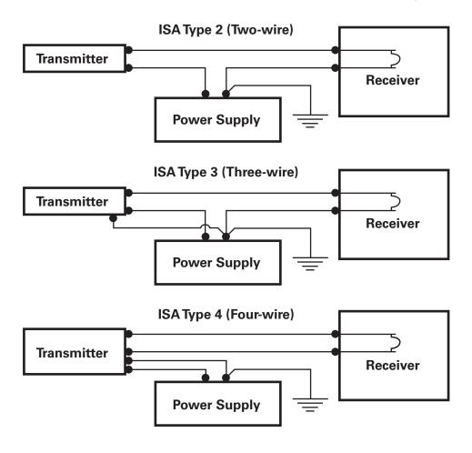
Figure 3-2. Typical 4-20 mA wiring
