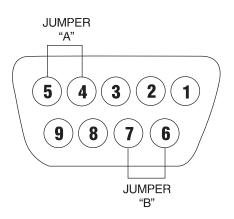
**Note:** Jumpers "A" and "B" are optional. See *page 3-3 External Inputs* for correct usage.
