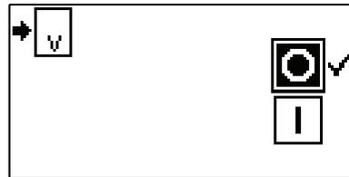
Using the UP and DOWN arrows on the control panel, highlight the
