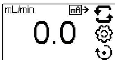
**NOTE:** When Current Output is selected the drive will not start until the CURRENT OUTPUT is ON and is in CONTINUOUS PUMP MODE.
