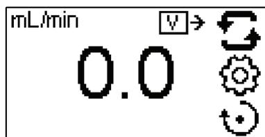
**NOTE:** When Voltage Output is selected the drive will not start until the VOLTAGE OUTPUT is ON and in CONTINUOUS PUMP MODE.
