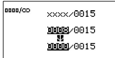
To reset the batch count, highlight the lower left and press ENTER.
