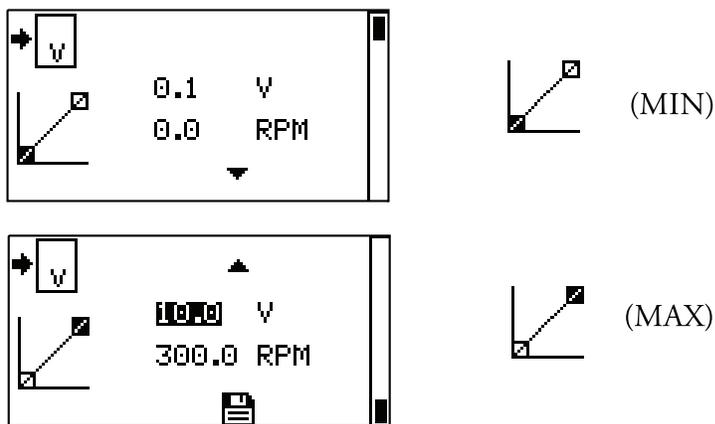
To confirm VOLTAGE INPUT MODE is ON, press the BACK key until the CONTINUOUS PUMP MODE screen appears. The Voltage input icon will be displayed.
