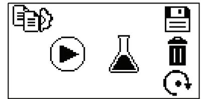
**SET COPY:** Press the START/RUN key on the control panel
