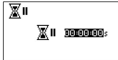
Using the UP and DOWN arrows on the control panel, highlight the time and press ENTER. The digits can be navigated individually using the UP/DOWN arrows; switch between digits by using the ENTER key. After selecting the Off Time, press ENTER again to validate. Press the back key to exit.
