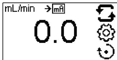
**NOTE:** When Current Input is selected the drive will not start until the CURRENT INPUT is ON and in CONTINUOUS PUMP MODE.
