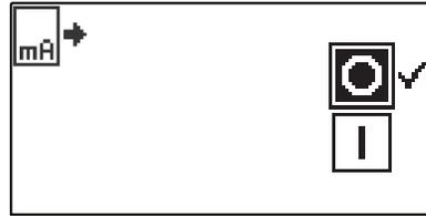
Using the UP and DOWN arrows on the control panel, highlight the  icon to activate, and press ENTER. A check mark ✓ will move next to it.
