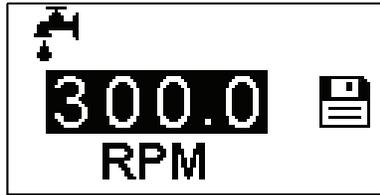
**FLOW RATE (RPM only):** When the entire rate field is highlighted, press ENTER. Press and hold the UP or DOWN key to change the RPM. The digits can also be navigated individually using the UP/DOWN arrows; switch between digits by using the ENTER key. After selecting an optimal flow rate, press ENTER again to validate. Press the back key to exit edit mode and save. (**NOTE:** RPM is the only unit available in Copy Mode.)
