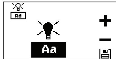
**DISPLAY CONTRAST:** This allows the user to adjust the contrast of the display for optimum viewing. By default the display is set for optimum viewing, using the UP and DOWN arrows on the control panel, highlight the **+** icon to increase the contrast or **-** icon to decrease the contrast, then press ENTER.
