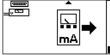
**CURRENT OUTPUT:** This allows the user to adjust the current output for a given flow. Press ENTER to Current output activation screen. By default the output is deactivated .
