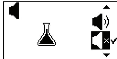
**DISPENSE SOUND:** This allows the user to have audio feedback when a dispense has completed. By default the sound is deactivated, using the UP and DOWN arrows on the control panel, highlight the
