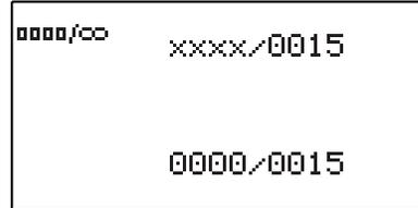
Using the UP and DOWN arrows on the control panel, highlight the top right number and press ENTER. The digits can be navigated individually using the UP/DOWN arrows; switch between digits by using the ENTER key. After selecting the batch count, press ENTER again to validate. If a batch count is not required, setting it to all 0000 will allow for continuous dispense cycling. This will also change the display icon to infinity ( $\infty$ ). Press the back key to exit.
