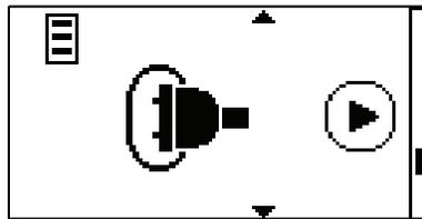
**DEFAULT SETTINGS:** Allows the drive to be reset to factory settings.
