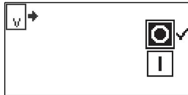
Using the UP and DOWN arrows on the control panel, highlight the
