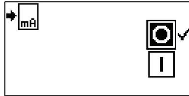
Using the UP and DOWN arrows on the control panel, highlight the
