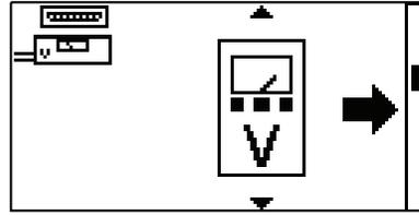
**VOLTAGE OUTPUT:** This allows the user to adjust the voltage output for a given flow. Press ENTER to Voltage output activation screen. By default the output is deactivated
