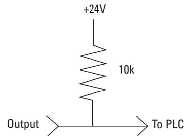
**Figure 3-11.** Terminating Open Collector Output to a PLC.
