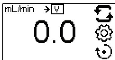
**NOTE:** When Voltage Input is selected the drive will not start until the VOLTAGE INPUT is ON and in CONTINUOUS PUMP MODE.
