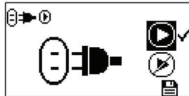
Using the UP and DOWN arrows on the control panel, highlight the
