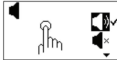
**KEY PRESS SOUND:** This allows the user to have audio feedback when a key is pressed. By default the sound is deactivated, using the UP and DOWN arrows on the control panel, highlight the
